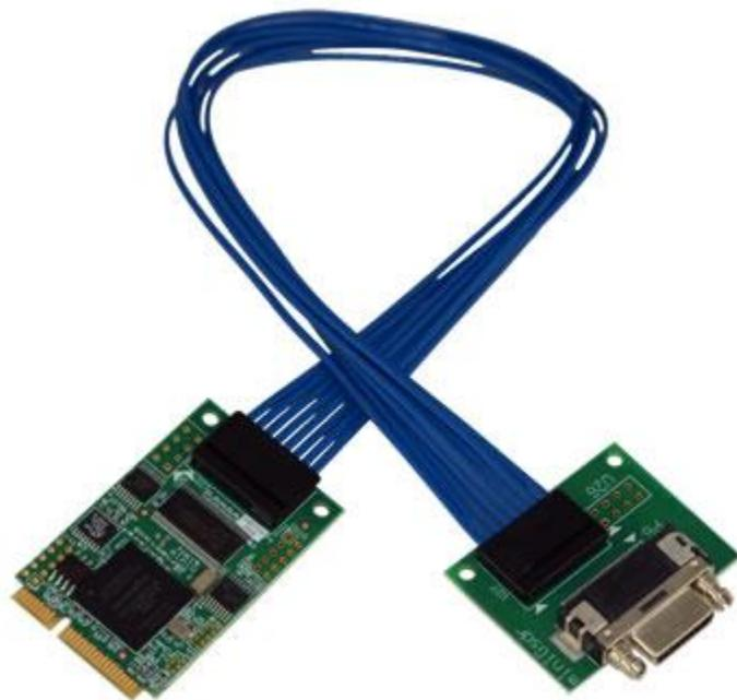
shown here with an SDR. At the maximum Camera Link clock rate of 85 MHz, a maximum length of 7 meters can be used.
