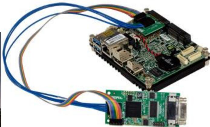
Half Mini Card standoff. This picture shows the PIXCI® EB1miniH with the MS-98H6 Motherboard. The motherboard supports Pentium and Celeron processors and has a Half Mini PCIe slot for the PIXCI EB1miniH. The motherboard has a Pico-ITX form factor measuring 100 x 72mm.
